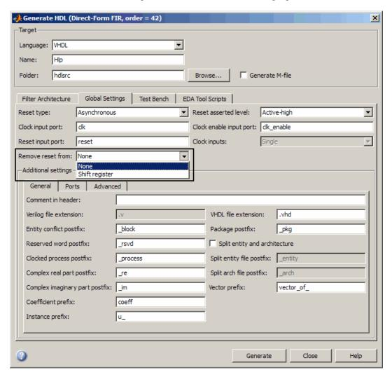
You can also use generatehdl function with the property RemoveResetFrom to suppress generation of resets from shift registers.
